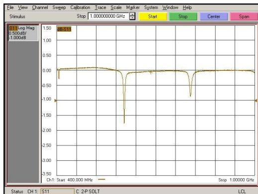
Fig. 21. S_{11} of manufactured TEM Cell without termination
