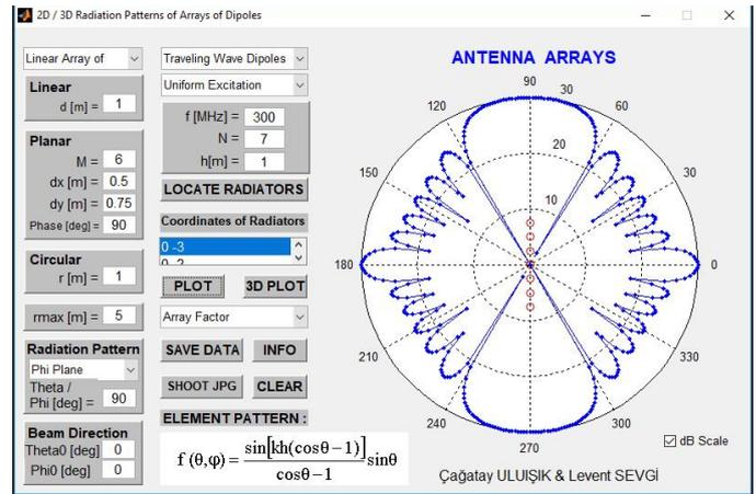
Fig. 3. The array factor of a linear array in a horizontal plane consisting seven elements excited uniformly ( $f=300$  MHz,  $d=1$  m).
