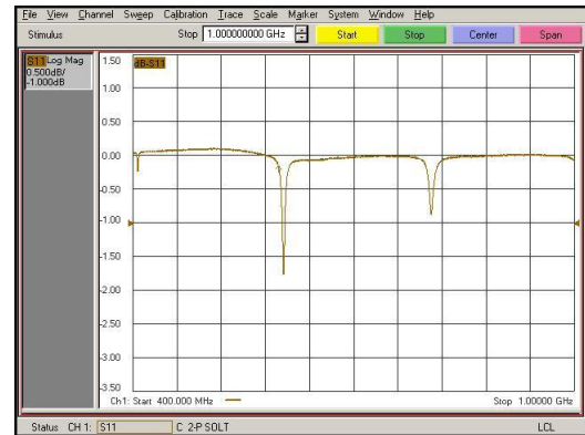
Fig. 23. S_{11} of manufactured TEM Cell
