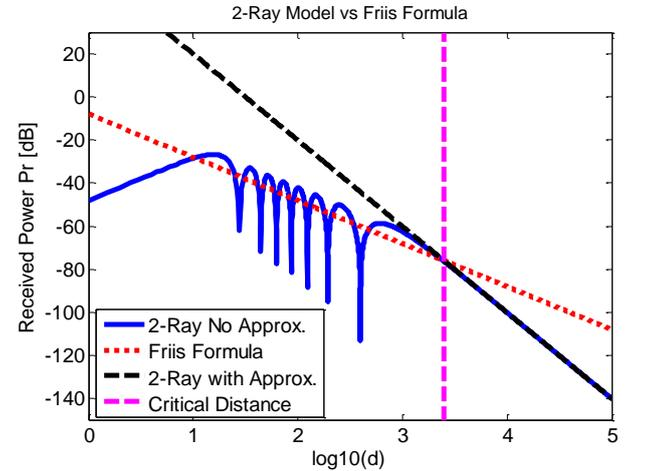
Fig. 5. The received power vs distance graph computed using the Friis formula and the 2-ray model ( $f=600$  MHz,  $P_t=100$  W,  $G_t = G_r = 1$ ,  $h_t=50$  m,  $h_r=2$  m).
