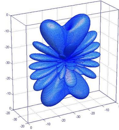
Fig. 2. The three-dimensional radiation pattern of a linear array consisting five standing wave dipoles ( $f=300$  MHz,  $d=0.5$  m,  $h=1.75$  m).
