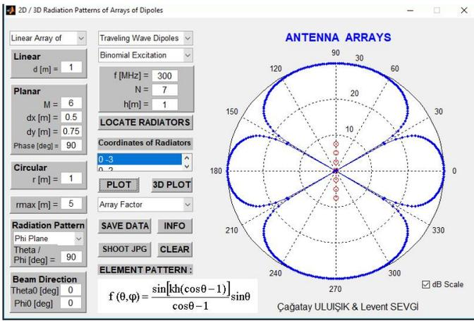
Fig. 4. The array factor of a linear array in a horizontal plane consisting seven elements excited binomially ( $f=300$  MHz,  $d=1$  m).
