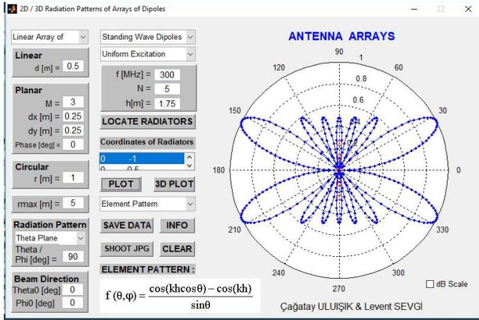
Fig. 1. The user interface of ArrayGUI. The vertical radiation pattern of a single standing wave dipole ( $f=300$  MHz,  $h=1.75$  m).
