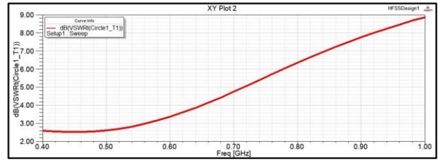
Fig. 15. VSWR of closed TEM Cell model – metal thickness 2 mm
