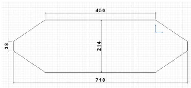
Fig. 4. Technical drawing of TEM Cell – top view (middle plate dimensions)
