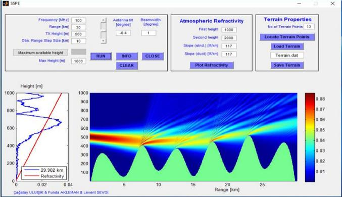
Fig. 6. The user interface of SSPE\_GUI.
